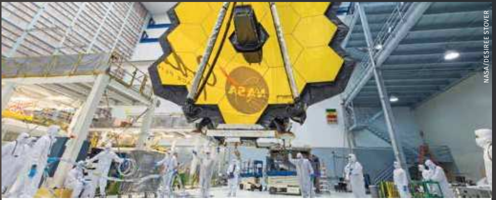
The James Webb Space Telescope's mirror hanging from the ceiling of a NASA warehouse. Workers in white coveralls are dwarfed standing beneath it. The mirror is composed of 18 hexagonal metallic gold-colored tiles.
